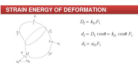
**Influence Coefficient**: The displacement at point 2 in a specified direction due to a force  $F_1$  applied at point 1 is proportional to  $F_1$ . The displacement produced at point 2 in a specified direction due to a unit force applied at point 1 is called **influence coefficient**  $a_{21}$ .
