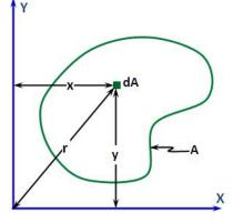
\*They are called so because of the similarity with integrals that define the mass moment of inertia of bodies in the field of dynamics. Since an area cannot have an inertia, the terminology moment of inertia of an area is a misnomer. This terminology for the above integral has become a common usage.
