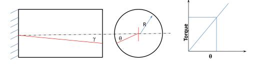
The relation between torque T and the angle of twist  $\theta$  is normally a straight line. Work done is the area under the torque angle graph. Strain Energy stored is given by  $\mathbf{U} = \frac{1}{2} \cdot \mathbf{T} \cdot \boldsymbol{\theta}$
