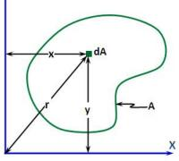
It is the moment of an area about an axis perpendicular to the x and y axis. Polar moment of inertia of an area is the sum of moment of inertia about x and y axis.
