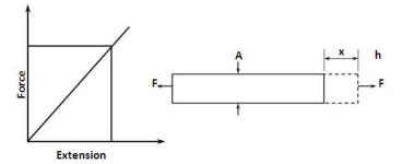
Consider a bar of length 'L' and cross sectional area 'A'. The bar is stretched when tensile forces are applied. The graph of Force versus extension is usually a straight line as shown in fig. When the force reaches a value 'F' the corresponding extension be 'x'
