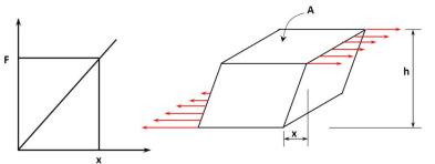
Consider the a rectangular element subjected to shear as shown in fig. above. The height is 'h' and the plan area is 'A'. It is distorted by a distance x due to shear force 'F'. The graph of force plotted against 'x' is normally a straight line, so long as the material remains linearly elastic.
